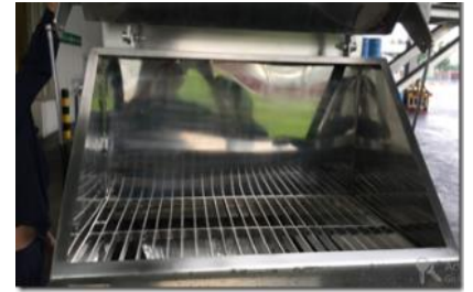
Inside Bag dumping station
